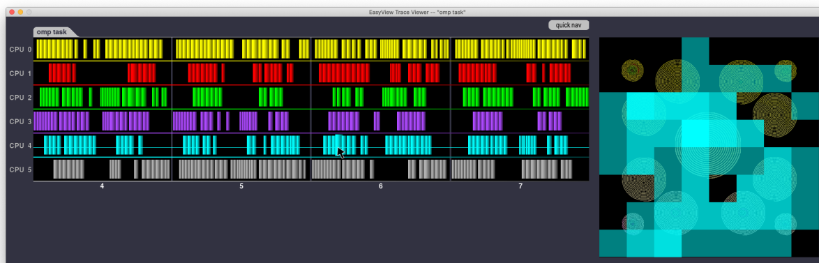
Figure 10: In horizontal mouse mode, it is possible to observe the set of tiles computed by a selected CPU. In this example, one can observe the spreading of tiles computed by CPU #4 during four iterations.
